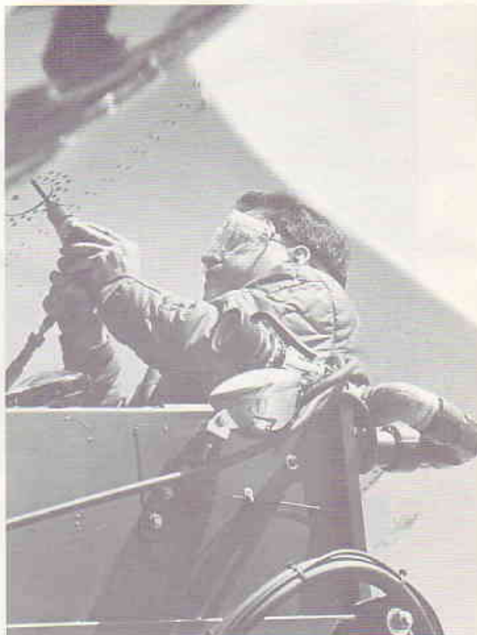
Drilling to Remove Stripped Screws from Tail Panel. SSgt. Timothy A. Gilbert stands in basket of cherry picker to get access to a part to be inspected. May 1987.
